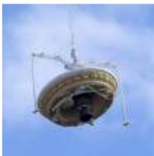
NASA has successfully conducted the first of three planned tests for the Low-Density Supersonic Decelerator project, developed to evaluate new landing technologies for future Mars missions.
